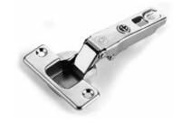
**ADJUSTMENTS (6-WAY):** 3mm to 6mm cup drilling distance range. -4mm horizontal adjustment. +2.5mm depth adjustment. Maximum overlay (3/4")
