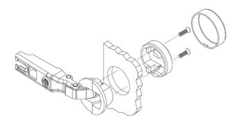
Mounting to glass door is obtained by means of a connecting ring that attaches to the hinge housing with two screws. The connecting ring and the screws are completely covered by an external face plate.
